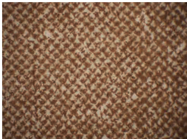
Figure 15a Detail of the print in fig. 14 (40x magnification), showing a typical rotogravure pattern.
