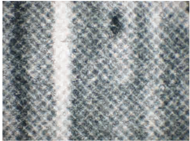
Figure 17a Detail of the print in fig. 16 (40× magnification). The rotogravure pattern is similar to that of other rotogravure prints.
