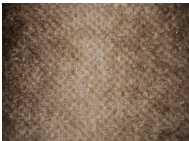
Figure 12a Microscopic detail of a rotogravure pattern in fig. 11 (40× magnification).
