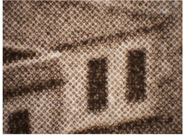
Figure 10b Microscopic pattern of a typical rotogravure print (25x magnification).
