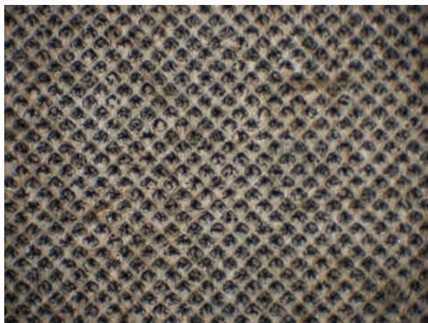
Figure 13b Detail of the rotogravure pattern in fig. 13a (40× magnification). Rougher stock caused some loss of detail in the Dmax areas.
