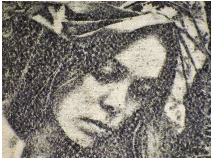
Figure 36a Detail of the polymer gravure print in fig. 34 (10× magnification), showing the use of a stochastic screen to create the gravure grain pattern on the plate.
