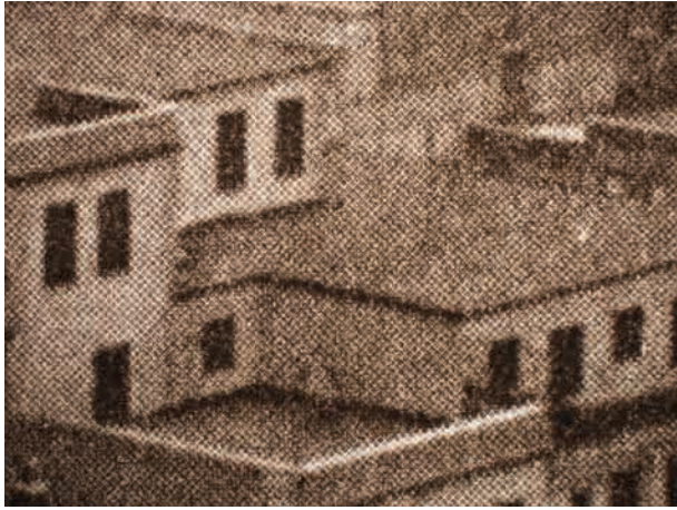
Figure 10a Microscopic pattern of a typical rotogravure print (10x magnification).
