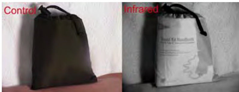
Figure 48 (above). The black material that this bag is made of is quite black in normal light (left) but almost transparent to infrared (right) - notice how clearly the writing can be read through the bag. This has been described, quite erroneously, as an 'x-ray effect.' Images © MaxMax.
