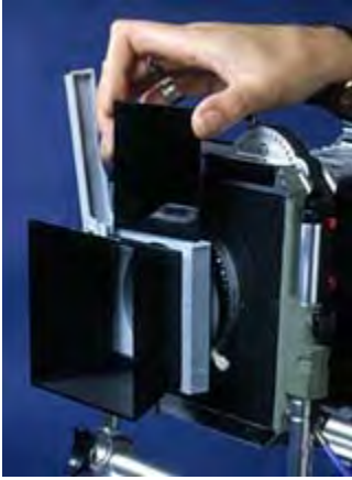
Figure 31 (left) - Kodak Pathe's Porte-filter Professional No.2 for large format work allows the visually opaque UV transmission filter to be dropped in after establishing the visual focus.
