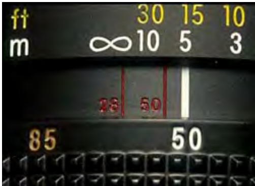
Figure 28. The infrared focusing marks often found on modern lenses. Two marks are actually engraved on this lens to represent the range of focal lengths of the zoom.
