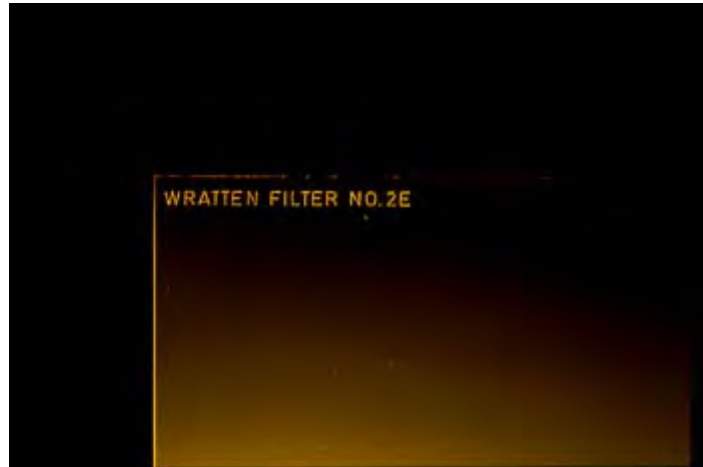
Figure 9 (above) - This fluorescence photograph of a Wratten 2E filter was taken with short wavelength radiation and a Wratten 15 barrier filter, and demonstrates that the Wratten 2E actually itself fluoresces. For critical work the barrier filter is therefore more effective if it is placed behind the lens: which then absorbs the shorter wavelengths of ultraviolet.
