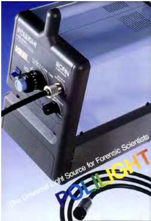
Figure 8 (left) - The Polilight has a series of stepped interference filters, which are then tunable by tilting their angle to the beam to give a continuously variable output from 300 to 1100nm.
