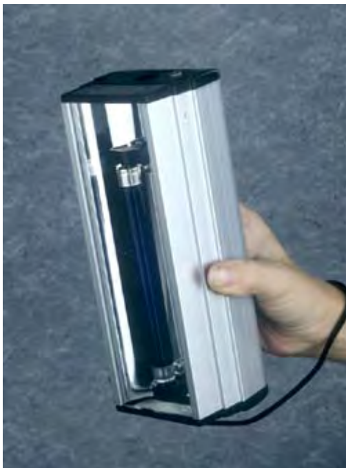
Figure 5 (left) - A battery operated, portable hand lamp is invaluable for identifying where (and if) fluorescence is occurring prior to full photographic recording
