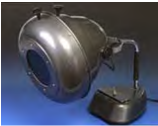
Figure 14 (left) - The 'classic' Wood's lamp found in many laboratories and clinics is a high pressure mercury vapor lamp fitted with a UV transmission filter - or Wood's filter - which effectively restricts the lamp's output to a single line spectrum at 365nm.
