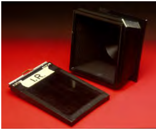
Figure 47 (left). Many materials transmit infrared freely despite their appearance in visible light this includes some plastics used for the manufacture of dark slides and camera bellows.
