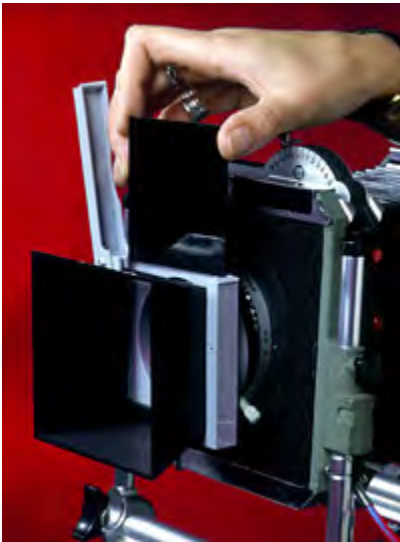
Figure 26. The Kodak Pathé filter holder designed so that the visually opaque filters can be quickly dropped into place.
