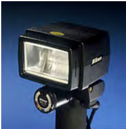
Figure 19 (left) - The Nikon SB-140 flashgun especially manufactured for invisible radiation photography with uncoated xenon tube and filters for visible, reflected ultraviolet and reflected infrared photography.
