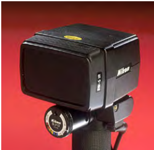
Figure 13. The Nikon SB-140 has a completely unfiltered tube with the facility to attach separate filters over the flash-head in light tight mounts: here we see it with the IR transmission filter in place.
