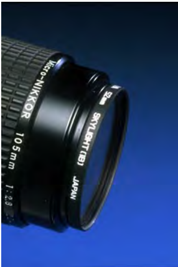
Figure 7 (left) - The 'UV Filter' or 'Skylight' filter routinely fitted to the front of camera lenses as physical protection is actually a UV blocking or barrier filter - useful for preventing the unwanted effects of haze in landscape photography and blue color casts in flash photography. It does not enable reflected ultraviolet photography but prevents it.
