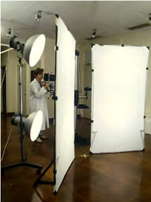
Figure 17. Lightform P22 panels in use to provide diffuse illumination for studio based infrared photography.
